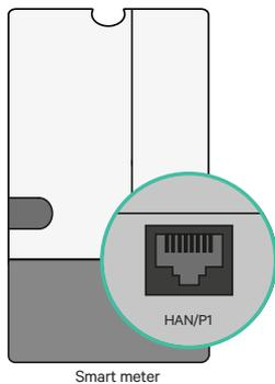
2. Fix the P1 Port meter to the DIN rail. Then, connect the RJ12 connector to the utility meter and the Wallbox P1 metering solution.
