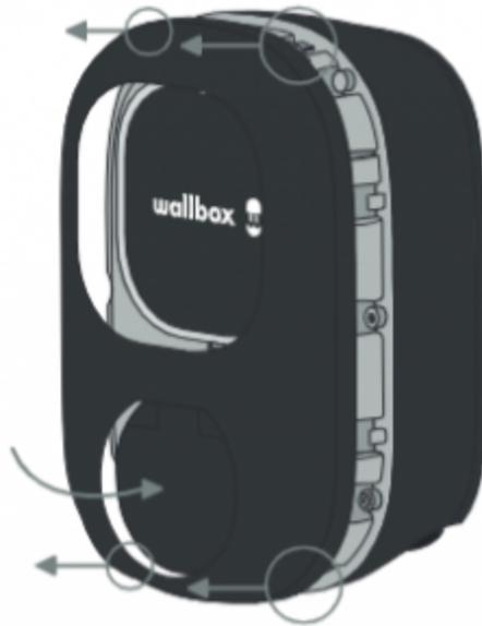
5. Unclip the style cover by pressing the socket lid with your fingers carefully.
