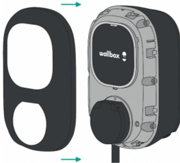
3. Clip back the cover frame on the charger and fix it with the other security screw. Do not over-tighten.
