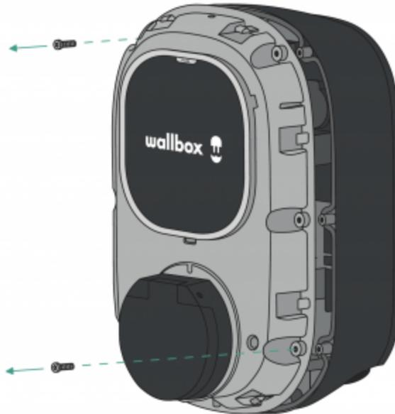
6. Remove the two corner screws and carefully lift the cover.
