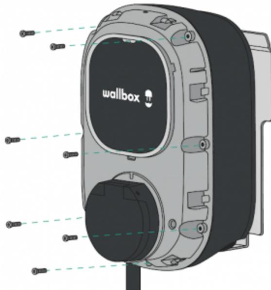
2. Insert seven corner screws to secure the charger cover. Do not over-tighten.
