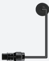
Plug and Play Cable is specifically designed for PV systems with a single microinverter. It consists of the field connector, AC cable, and plug. The field connector is connected to the microinverter connector, and the plug is connected to the household socket in accordance with local regulations.
